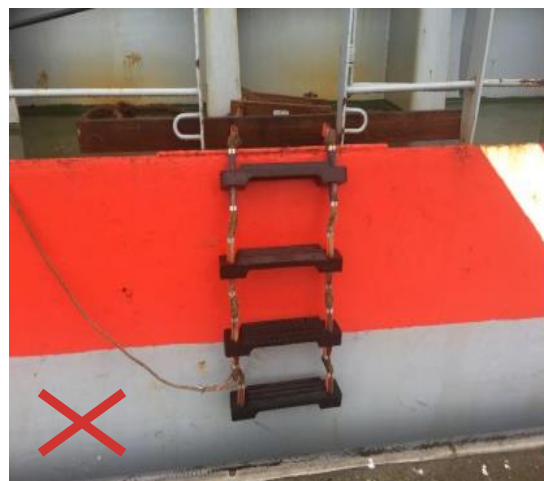
Spreader used for securing & tripping line secured (must be over the 1st spreader from bottom and leading in the forward direction)
