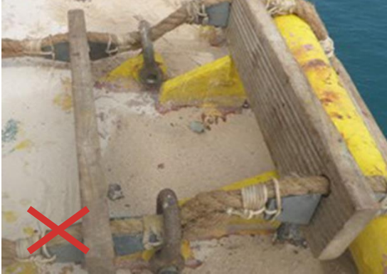
Secured using shackles, risk of damage to the chocks
