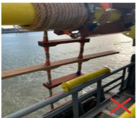
Ladder on the reel & not secured incorrectly rigged
