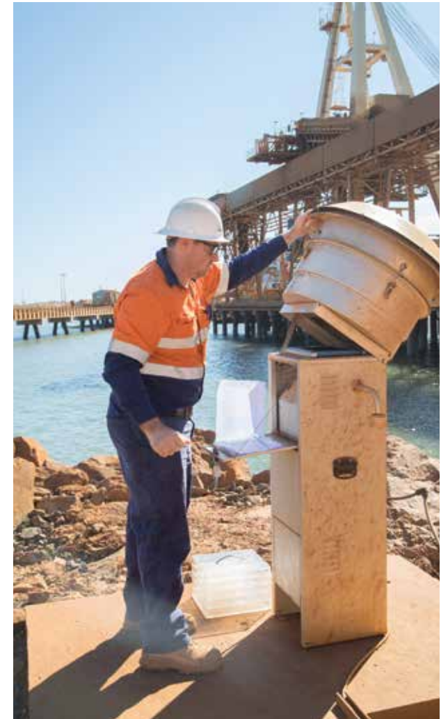
Environment Advisor Jakeb Cumming checks one of the dust monitors at Utah Point Bulk Handling Facility at Port Hedland.
