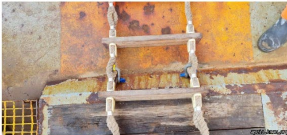
Photo 5: Unsafe pilot ladder securing arrangements.
