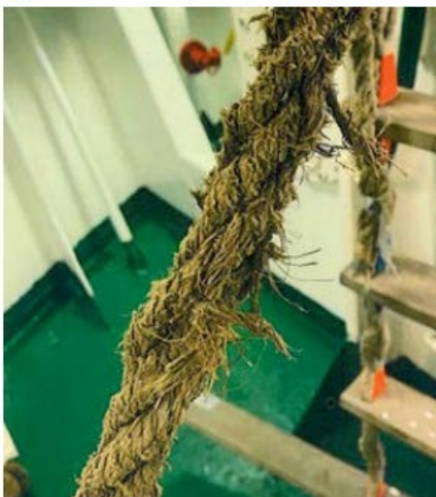
Photo 10: Frayed side rope.
